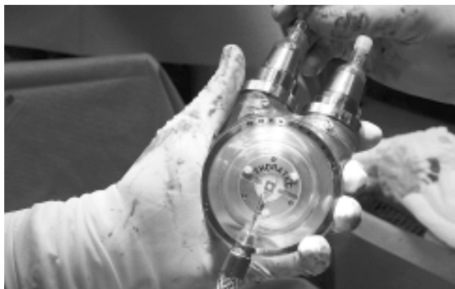
Fig. 2. Detail of the pumping chambers, either of them replacing function of one heart ventricle
