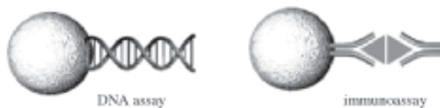
Fig. 1. The LabMAP Luminex technology uses 5.6 micron polystyrene microspheres which are internally dyed with fluorophores. Probes are bound to surface through carboxyl groups or avidin.
